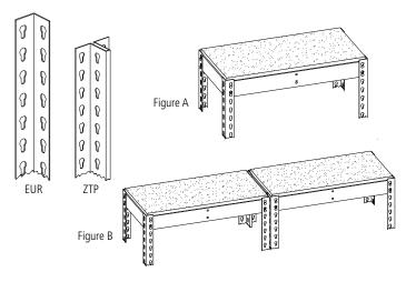
**3.** With the help from an associate, or using a wall for support, connect two EUR uprights (Ref. No. 1) using two front-to-back supports (Ref. No. 3), one at the top and one near the bottom (leaving the bottom-most keyhole slot empty). Be sure the front-to-back supports are fully seated in the keyhole slots as shown.
