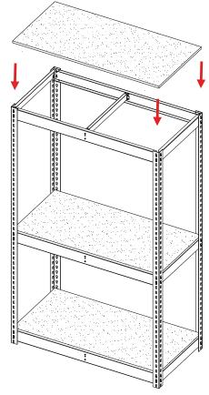
**9.** If joining more than one unit together, your original unit should have been assembled with ZTP uprights on one end, as described in step 4. Simply continue adding shelf supports and uprights to complete your additional units.
