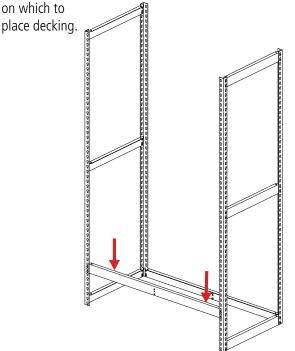
**6.** Attach the remaining shelf supports at the desired shelf levels, making sure that all shelf supports are completely seated in the upright slots.
