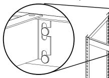
NOTE: Recommended number of reinforements per shelf are as follows: 48"w-69"w = 1 reinforcement 72"w = 2 reinforcement 84"w-96"w = 3 reinforcements
