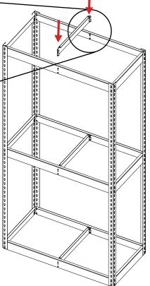
**8.** If particle board decking (Ref. No. 6) was ordered, place the decking on each shelving level. The decking should fit flush inside the shelf supports. If you have purchased a single unit, your shelving unit is now complete. For adder units, see step 9.
